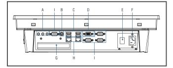
A: Line in/Line out/Mic in B: PS2 Mouse & Keyboard C: USB 2.0 x 4 D: VGA Port E: Power Switch F: AC Inlet G: PCI Slot x 1 H: 10/100/1000 Base-T Ethernet x 2 I: RS-232 x 3, RS-232/422/485 x 1
